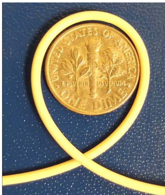
Figure 6. Image of a flexible PAI/silica hollow fiber sorbent [minimum radius (Dime) 9 mm]. [Color figure can be viewed in the online issue, which is available at wileyonlinelibrary.com .]
